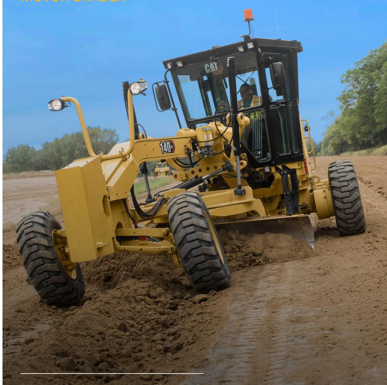
Engine Power Operating Weight 131 kW-147 kW (176 hp-196 hp) 18 365 kg (40,488 lb)
