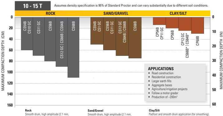
Smooth drum, high amplitude (2.1 mm, 0.083 in) moving to low amplitude when approaching compaction, 4-8 passes Smooth drum, high amplitude (2.1 mm, 0.083 in) moving to low amplitude when approaching compaction, 4-6 passes
